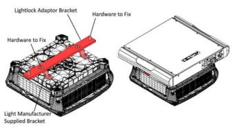
Alternatively you can rig the moving light from a 50mm / 2'' diameter pipe which is clamped below the RSC Lightlock unit via 2 half couplers fitted to the bottom slots of the RSC Lightlock using M12 / 1/2'' screws.
