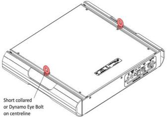
**2 way Bridle assembly:** Fit hard eye ends of 2 way bridle to slots in bridle bracket. Remove security screw. Slide bridle bracket into top slot and refit security screw. Repeat for other side. Fit shackle between delta ring and suspension eye.
