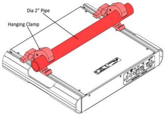
On top of 50mm / 2" pipe diameter pipe: Fit 2 half couplers to bottom slots of RSC Lightlock using M12 / 1/2" Screws.
