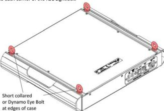
**2 wire hang:** Fit 2-M12/1/2" full nuts into top slot. Fit M12/1/2" Short Collared or Dynamo eye bolts and washers into M12/1/2" nuts and secure to centre of the RSC Lightlock.
